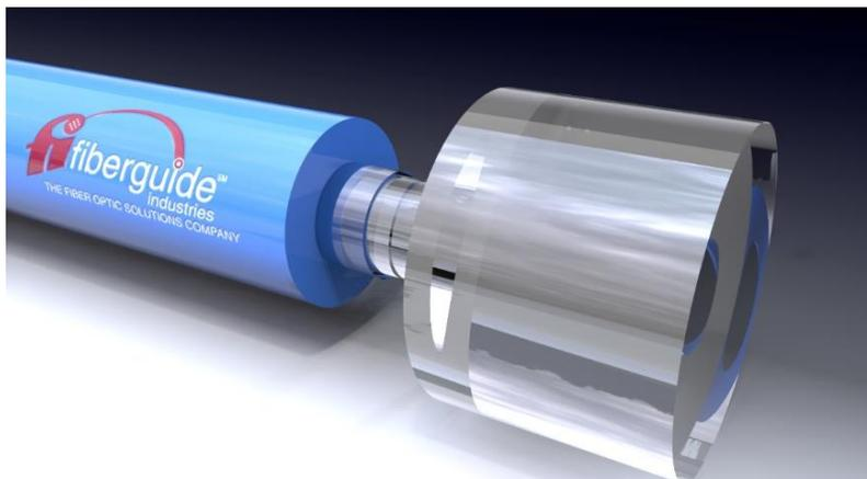
Fiberguide's end capped fiber optic assemblies allow the user to achieve higher coupled power into a fiber core by reducing the power density at the air/ silica interface, commonly the point of laser damage. End cap diameters and lengths are offered for select numerical apertures and fiber cores size, but can be easily customized for a variety of fiber types and specialized applications.
