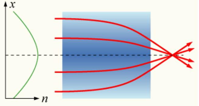
Figure 1: Graded Index Lens (Example)
