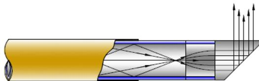
Figure 2: OCT Probe With Side Fire Tip
