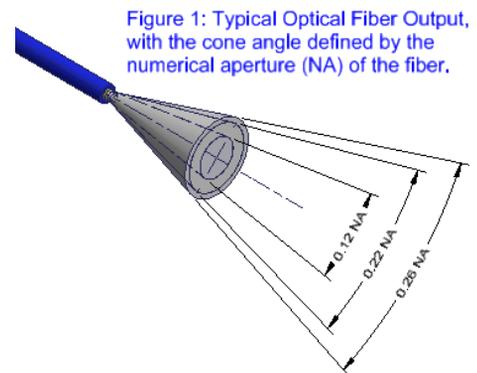
Figure 1: Typical Optical Fiber Output, with the cone angle defined by the numerical aperture (NA) of the fiber.
